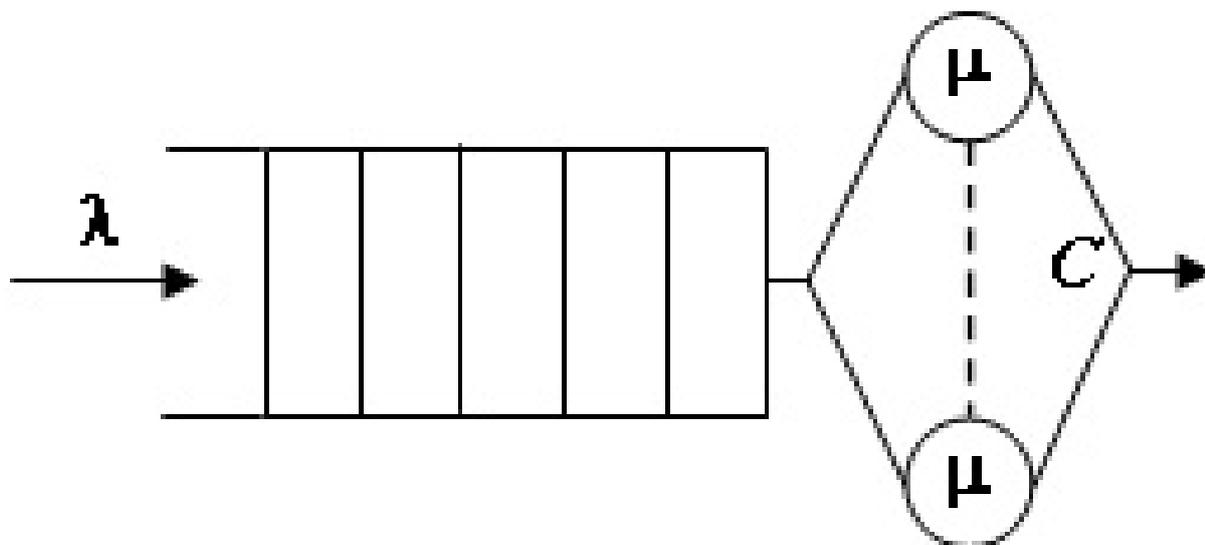
FIGURE 2.8 – La file  $M/M/C$
