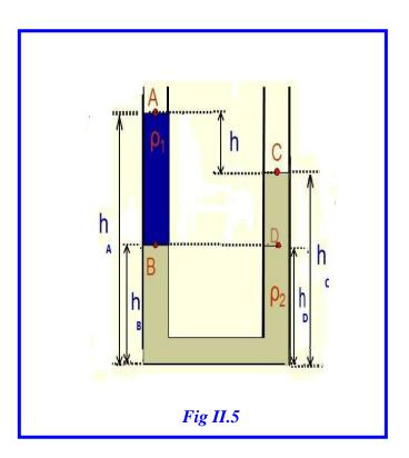
$$\begin{cases} p_D = p_{atm} + \rho_B g(h_B - h_D) \\ p_C = p_{atm} + \rho_A g(h_A - h_C) \end{cases} \Rightarrow p_{atm} + \rho_B g(h_B - h_D) = p_{atm} + \rho_A g(h_A - h_C)$$
