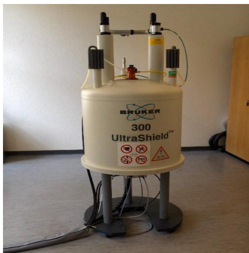
Figure B-1-8 :appareil RMN de type BRUCKER AM (300MHz).
