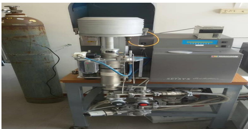
Figure 2.19: Installation of thermal measurements (TGA-DTA) by Setaram Setsys 1200 TG.
